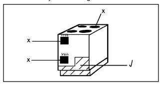
To move the appliance, open the main oven door, and lift the appliance by holding inside the top of the compartment.
